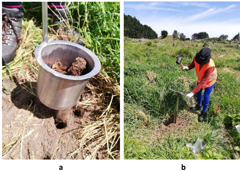
Figure 4-2 Soil sampling; (a) a bucket soil sampler to collect samples from 0-10 cm depth, and (b) a soil auger to obtain samples from 30-45 cm depth.
